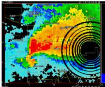
The interpolation scheme in the vertical between adjacent beam centerlines, and is not an image smoothing technique. This is important for the CAPPI cross-sections since there can be significant gaps in coverage. These gaps are filled in be data just above and below these gaps. If they were filled in from the "sides" (horizontally), significant visualization errors would result.
