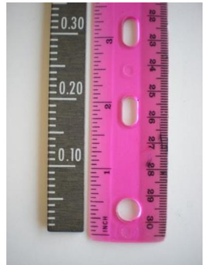
Figure A-5. The Measuring Stick (brown) for Eight-Inch Gauge.
