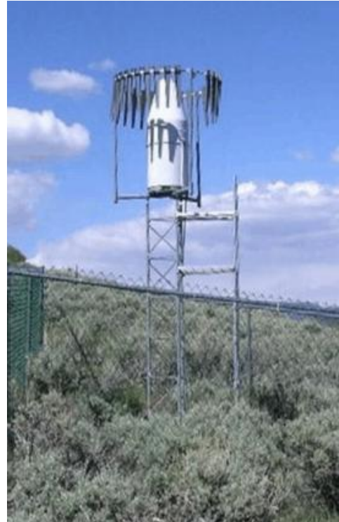
Figure A-3. Fischer-Porter Gauge on a Snow Tower with Wind Shield.
