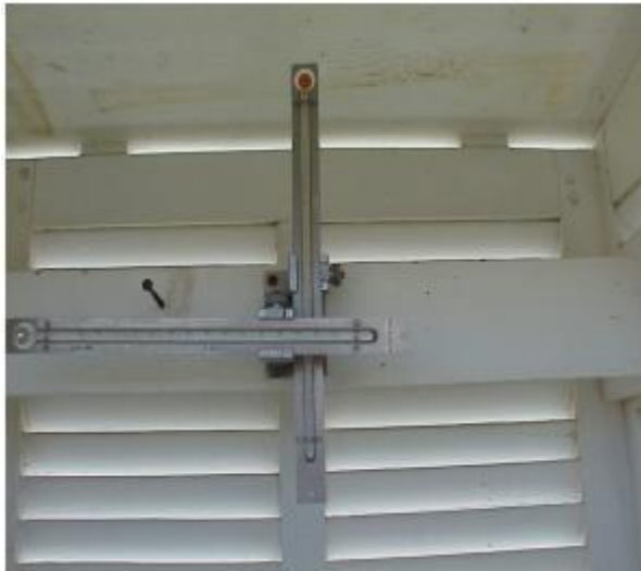
Figure B-30. Minimum Thermometer – Vertical Position During Resetting
