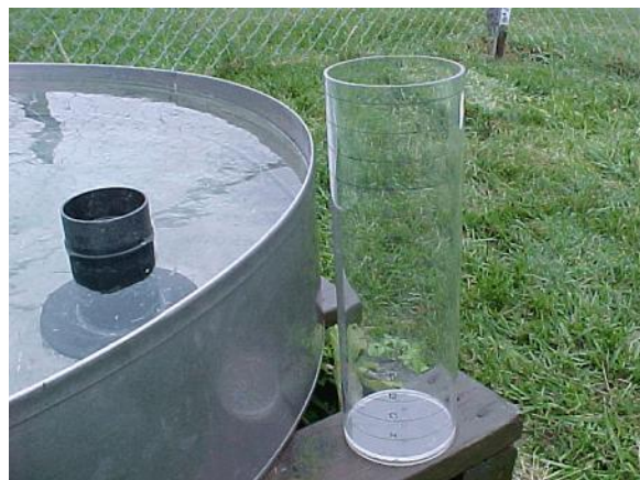
Figure B-36. Transparent Measuring Tube and Stilling Well Inside the Pan
