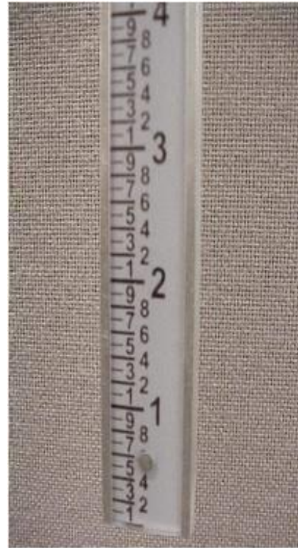
Figure B-16. Snow Sticks Measure in Tenths of an Inch
