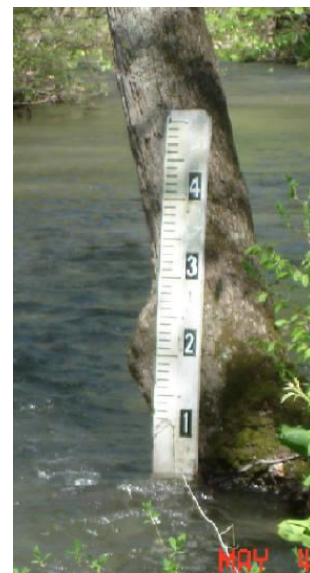
Figure B-50 – Reading the Staff Gauge
