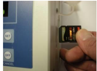
Figure B-21. Insert SD Memory Card to Download Last 60 Days
