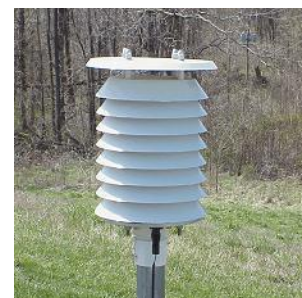
Figure A-14. MMTS Shelter
