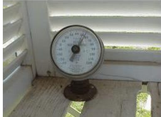
Figure A-35. Palmer Soil Thermometer Display in Shelter
