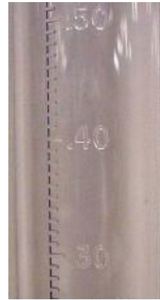
Figure A-8. Measuring Tube is Marked in Hundredths of an Inch
