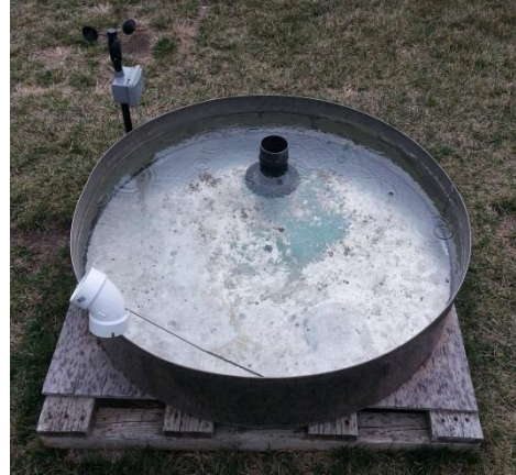
Figure A-32. Position the Long Stem Probe into Shaded Side of Pan
