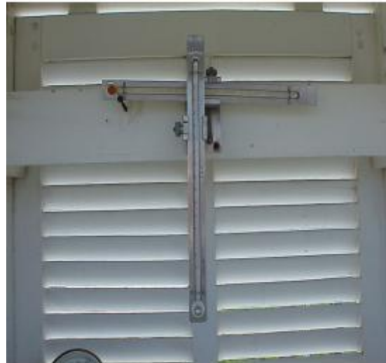
Figure B-31. Maximum Thermometer in Reading Position
