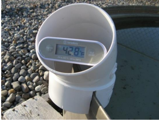
Figure A-31. PVC Holder for Long Stem Digital Thermometer
