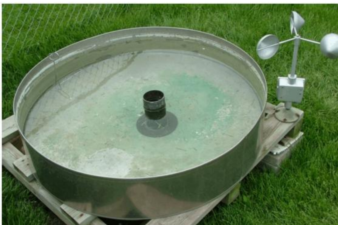
Figure A-23. Evaporation Pan with Stilling Well and Totalizing Anemometer.
