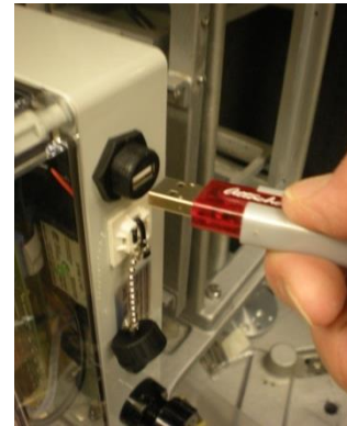
Figure B-24. Insert Flash Drive to Download Last 100 Days
