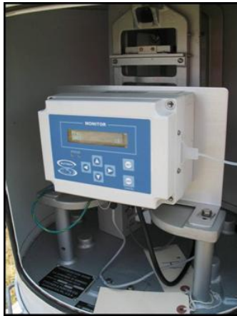
Figure B-20. FPR-D Data Logger
