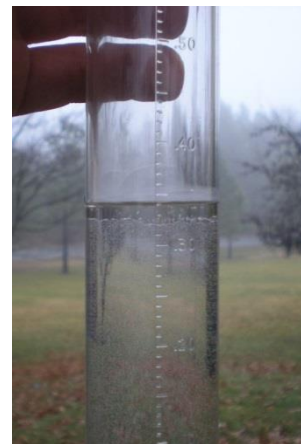
Figure B-7. Reading the Measuring Tube at Eye Level
