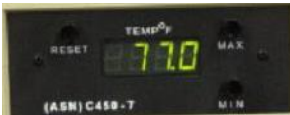
Figure B-26. MMTS Control Buttons
