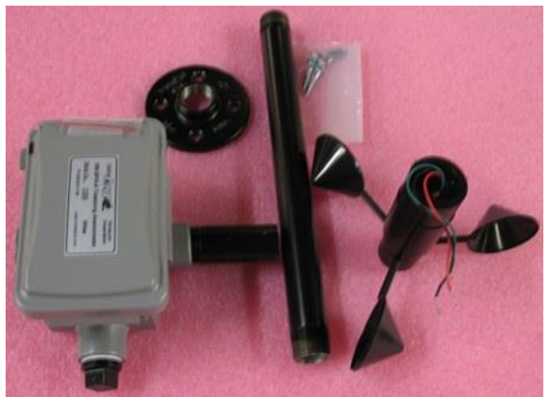
Figure A-28. Totalizing Anemometer (ASN Part F106-1)
