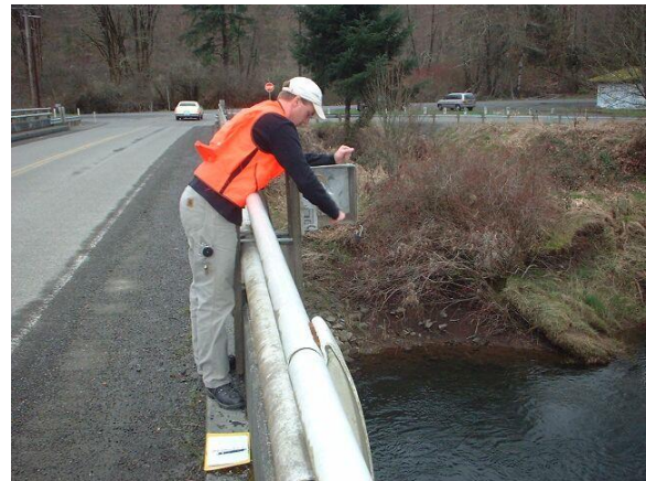
Figure B-46 – Observer at Wire Weight Gauge
