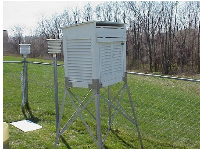
Figure A-13. Instrument Shelters: Cotton Region Shelter and Two MMTS Shelters
