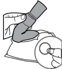
Figure C-11: Inserting the Nozzle Ring
