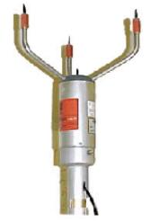
Figure J-3: Vaisala Handar Wind Sensor
