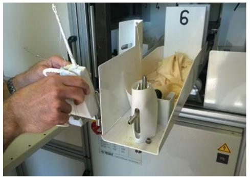
Figure C-18: Placing the Radiosonde in the Holder
