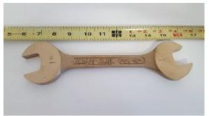
Figure K-15: Typical Brass Non-Sparking Wrench
