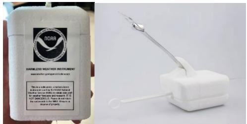
Figure A-1: Upper Air Radiosonde (GRAW)
