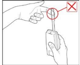
Figure C-14: Do not Touch the Radiosonde Sensors
