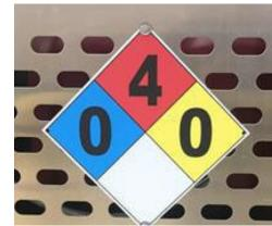
Figure K-12: NFPA 704 Placard for Hydrogen
