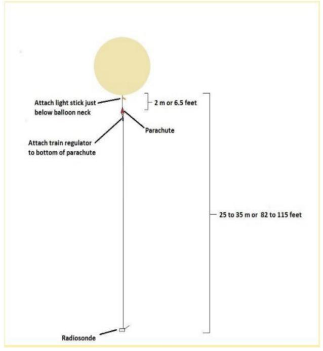
Figure A-7: NWS Radiosonde Flight Train
