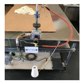
*Figure K- 4 - Typical Fill Valve with approved hose to nozzle, 1/4 turn isolation valve, fill pressure gauge, stainless steel grounded table, and classified fill controller/solenoid*
