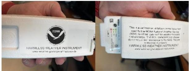
Figure A-2: Upper Air Radiosonde (Vaisala)
