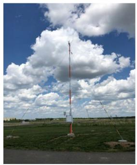
Figure J-10: Automatic Weather Station (AWS)
