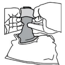
Figure C-12: Folding the Balloon Neck over the Ring
