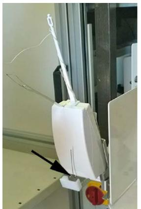
Figure C-19: Correct Placement of the Radiosonde Antenna
