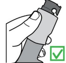
Figure C-13: Balloon Neck Correctly Folded over the Ring
