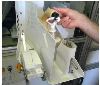
Figure C-22: Unwinder Hook Attached to the Balloon Nozzle
