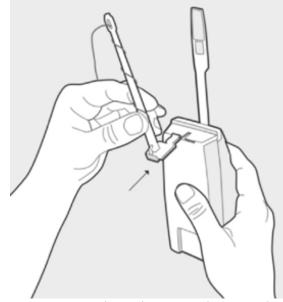
*Figure C-15: Pushing the Unwinder into Place*
