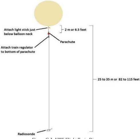
Figure C-3: NWS Flight Train Diagram
