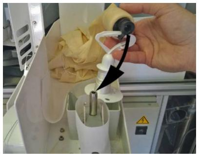
Figure C-23: Snapping the Nozzle on the Nozzle Pipe
