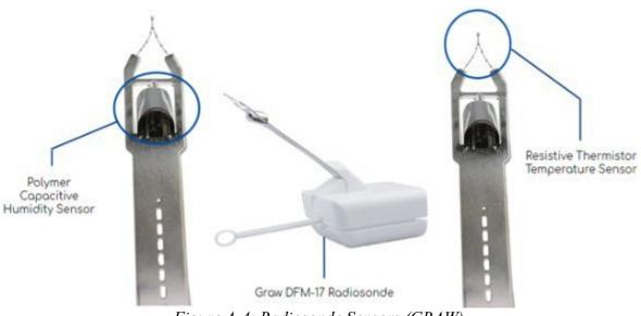
Figure A-4: Radiosonde Sensors (GRAW)
