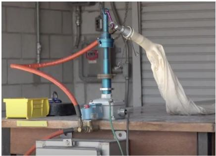
Figure C-1: Balloon on Inflation Table Secured w/Clamp
