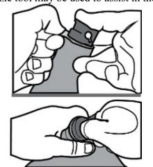
Figure C-10: Inserting Balloon Nozzle on the Balloon Neck
