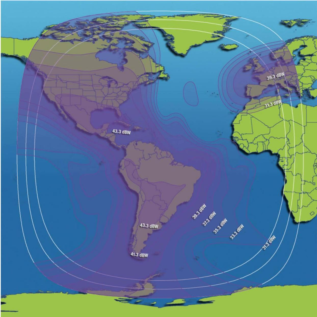
IntelSat 21 GNC-A C-band broadcast earth coverage and signal strength.
